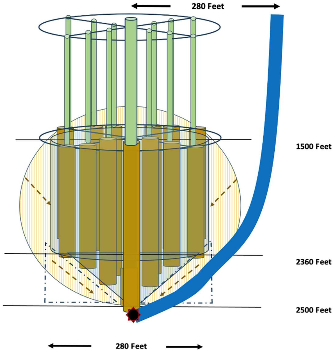
Figure 1: Proposed HBHM initial layout at Bonnie Claire. Wells (brown cylinders) are centered and spaced within a 280-foot diameter surveyed section. Slurry is hydraulically airlifted to a single directionally-drilled Production Well offset from Mined section center (Blue cylinder). Note: the figure depicts 13 wells for illustrative purposes. Actual modelling is based on 32 wells.
