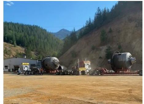
Photo 6: Ball mills arriving by lowboy trailer at Bunker Hill
