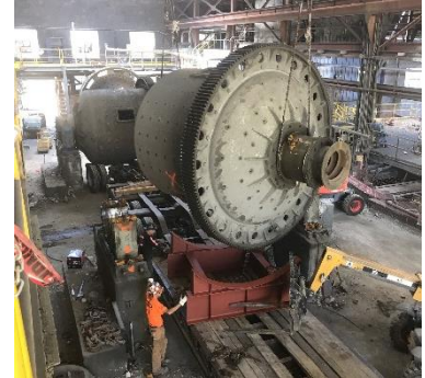
Photo 3: Ball mill loaded on trailer
